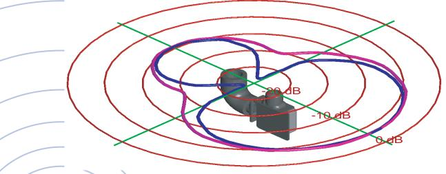
**Figure 2**: FP microphone measured free-field response at 2kHz (magenta) vs. ideal limaçon curve (blue)
